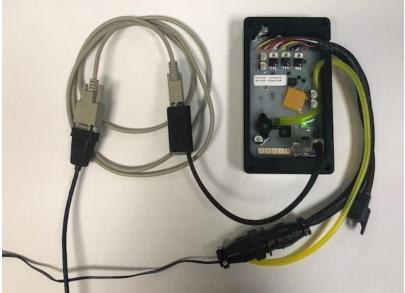
CONNECT SERIAL TO SERIAL TO COMPUTER (USE DB9 USB/SERIAL ADAPTER for COMPUTER W/O SERIAL PORT)
